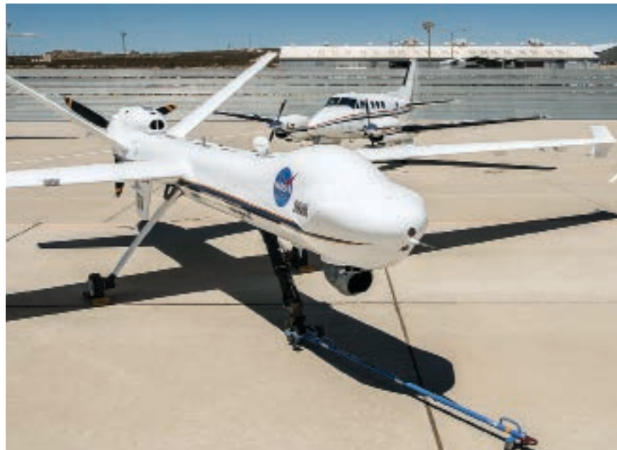
At Edwards Air Force Base in California, NASA has been conducting flight tests with a General Atomics MQ-9 UAV (foreground) and a Beech King Air (rear), which flies intrusions into the Reaper’s path.
