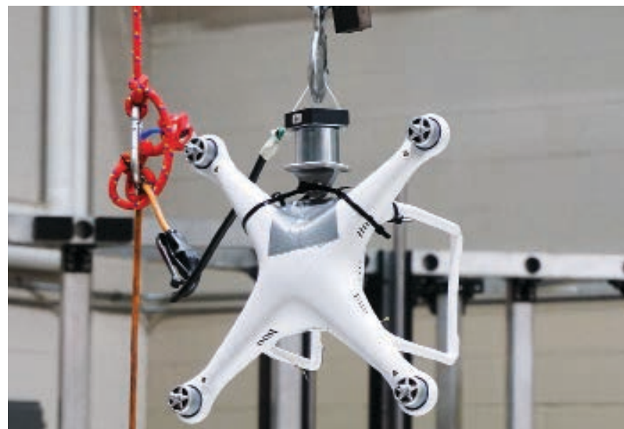
The National Institute for Aviation Research is also investigating the damage potential of collisions between UAVs and airplanes by crashing quadcopters (above) into the materials used to build airframes.
