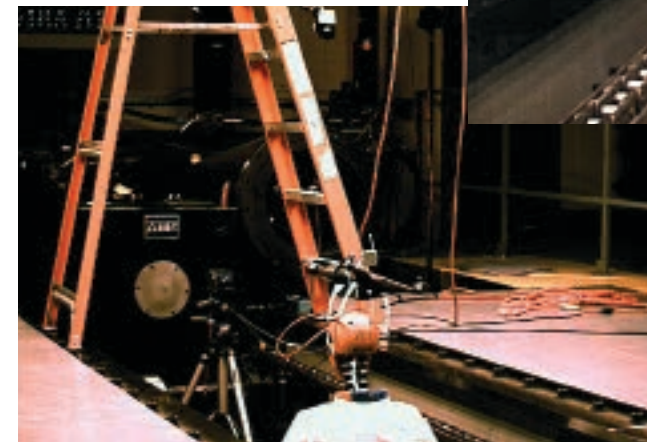
If a UAV falls out of the sky and crashes into a person's head, what injuries could result? Researchers at Wichita State University's National Institute for Aviation Research are trying to find out by dropping drones onto test dummies.
